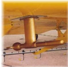
**Inertial Measurement Unit (IMU):** The AIMMS-20AG inertial module is a full six-degree of freedom IMU containing three rate gyros and three accelerometers. Angular rates and accelerations are broadcast 40 times a second in order to precisely track the dynamics of the aircraft attitude over the complete flight envelope.
